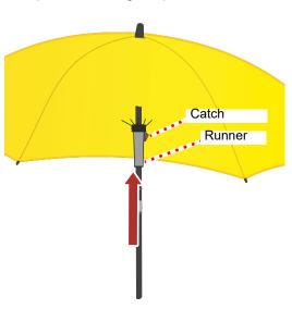
Keep parasol away from you, press catch and push slider upwards. The parasol spreads out and the slider engages in the upper position.
